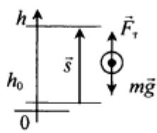
$$\begin{aligned} A &= F_s \cos \alpha, \\ \vec{F}_t &\uparrow\uparrow \vec{s}; \quad \cos \alpha = 1, \\ F_t &= mg; \quad s = h - h_0, \\ A &= mg(h - h_0) = \Delta E_p. \end{aligned}$$
